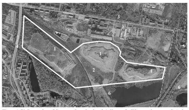
**Figure 1.** Bird's-eye view of the area to be redeveloped. 1. Heaps of solid excavation waste, 2. Active railway line no. 132, 3. national road 94, 4 national road 79, 5 Administrative border of Bytom and Chorzów, 6. "Żabie Doły" nature and landscape complex (own elaboration based on Geoportal Bytom, 2020).
