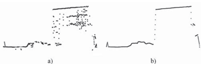
Fig. 4. A sample set of points (a) located in two-dimensional space is processed by the envelope filter, resulting in a point set (b) representing the outer surface of the object
