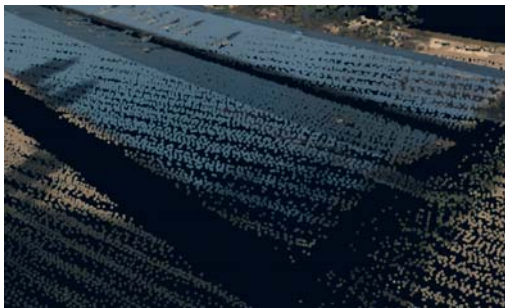
Fig. 1. Sample dense point cloud representing a set of buildings of relatively simple shape. Image captured with a visualization application created by one of the authors
