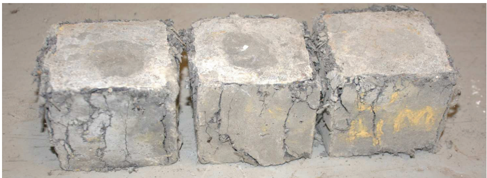
Figure 4. Typical failure pattern of ECC cubes
