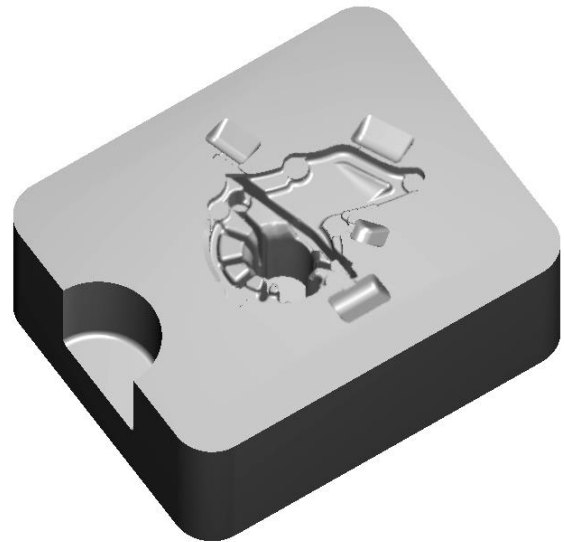
Fig. 8. Real model of movable die insert after machining
