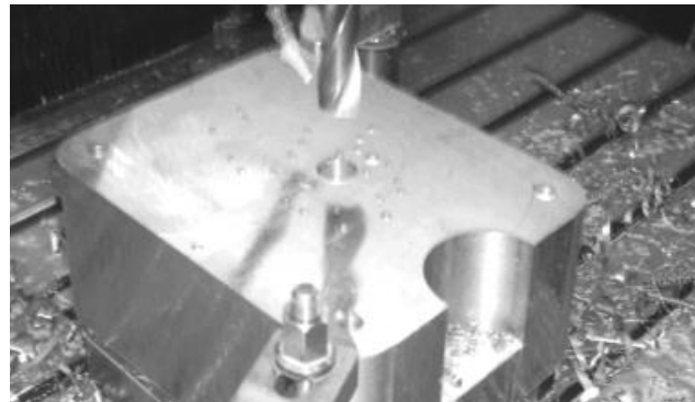
Fig. 3. Hole drilling in movable die insert on jig drilling machine
