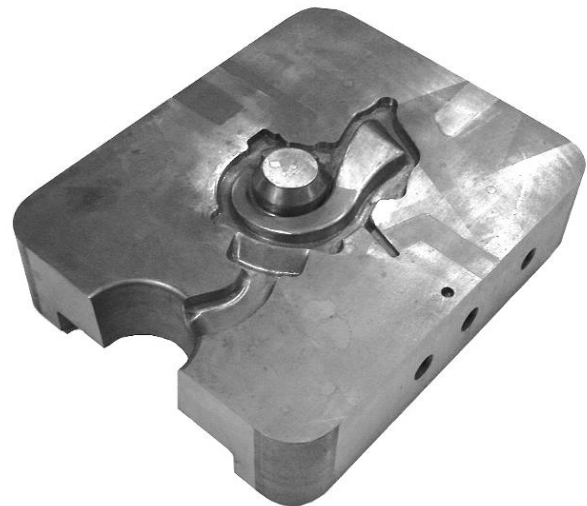
Fig. 9. Real view of fixed die insert after machining
