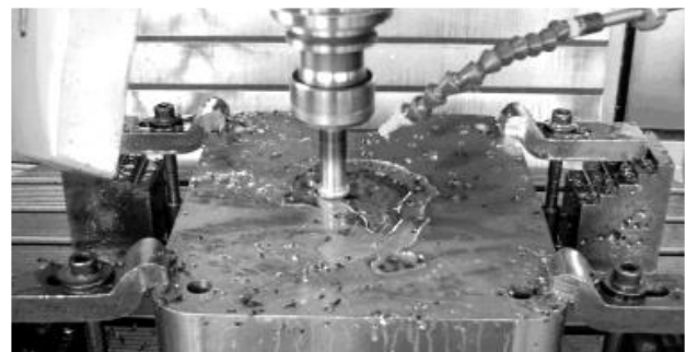
Fig. 4. Rough milling of movable die insert shape
