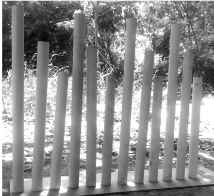
Fig. 1. Concrete filled steel tubular specimens
