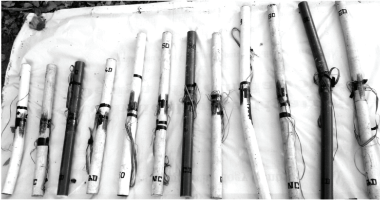
Fig. 3. Tested concrete filled tubular columns
