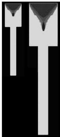
Fig. 5. Shrinkage defects obtained from simulations of steel casting solidification; the smaller plate dimensions (thickness x width x height, in mm) are: 30 x 150 x 280 (left) and 60 x 240 x 520 (right)
