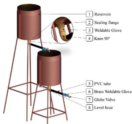
Figure 8. Schematic representation of the experimental module made. 1 – Brass reservoir with capacity of 20 L; 2 – PVC flange of 1 1/4"; 3 – PVC weldable glove of 3/4"; 4 – Knee 90° PVC of 3/4"; 5 – All PVC of 3/4"; 6 – 3/4" weldable sleeve/brass thread; 7 – 3/4" globe valve (tap); and, 8 – 5/16" transparent polyethylene level hose for visual monitoring of the liquid level in the tanks
