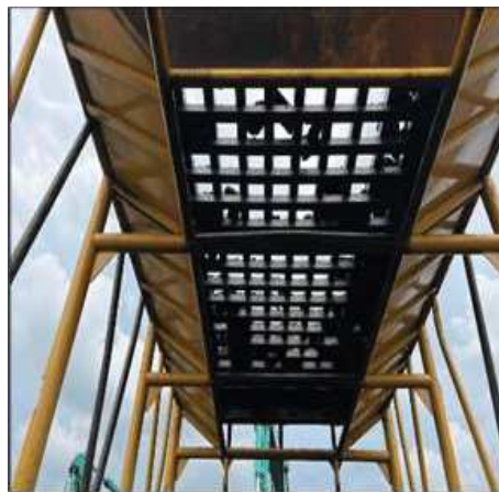
Fig. 6. Coal Stuck in the Sidelines of Fixed Screen
