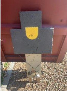
Photo 3. Contact target with two pieces of mesh separated by foam, with foam support
