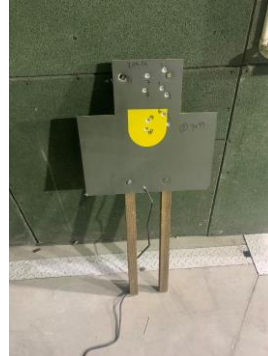
Photo 4. Contact target with two aluminium sheet metals separated by form, with wooden legs
