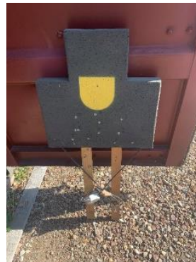
Photo 2. Contact target with two pieces of mesh separated by foam, with wooden legs
