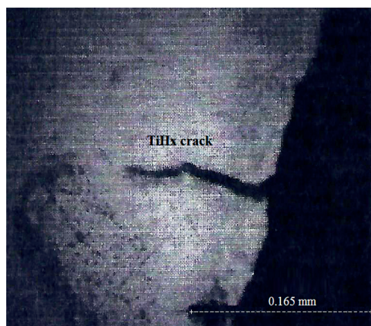
Fig. 16. Microstructure of sample S2 following immersion in H_2SO_4 (0.1 M), using J = 100 \text{ mA/m}^2 , during 72 hours
