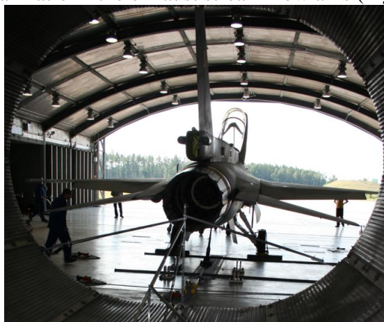
Fig. 12: Positioning of the probe in the axis of the exhaust stream from the engine outlet nozzle
