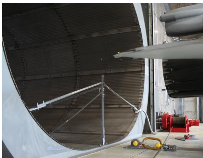
Fig. 2. Exhaust sampling probe mounting location
