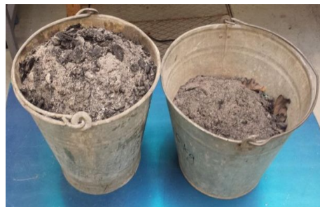
Fig. 4. Ash with visible fragments of incompletely combusted fuel
