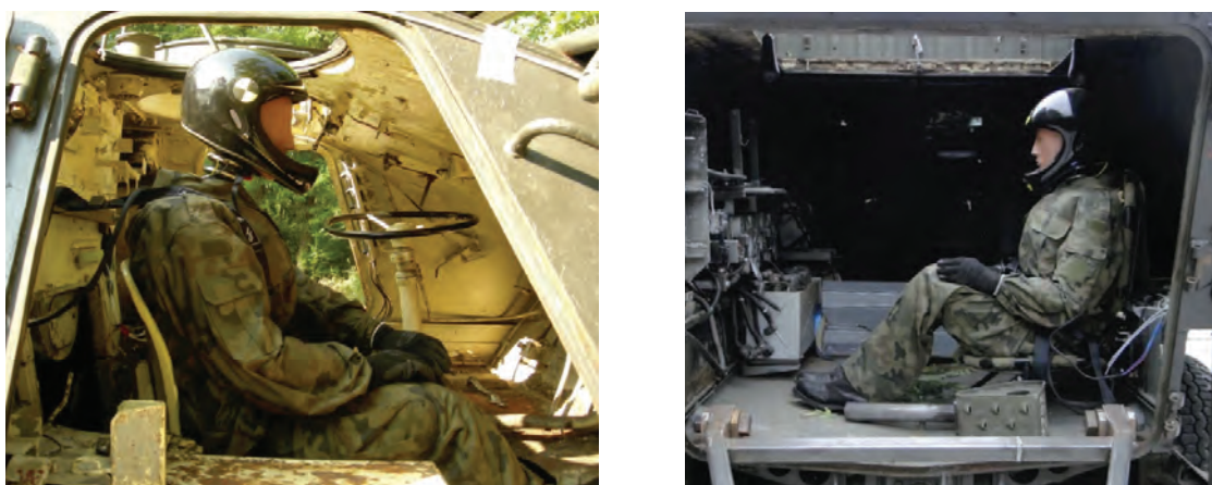
Fig. 2. A dummy located in the driver compartment (left) and in the landing troop compartment (right)
