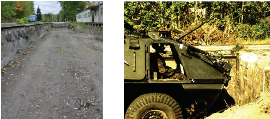
Fig. 1. The view of a test track with a rigid retaining wall and a personnel carrier prepared for a crash test
