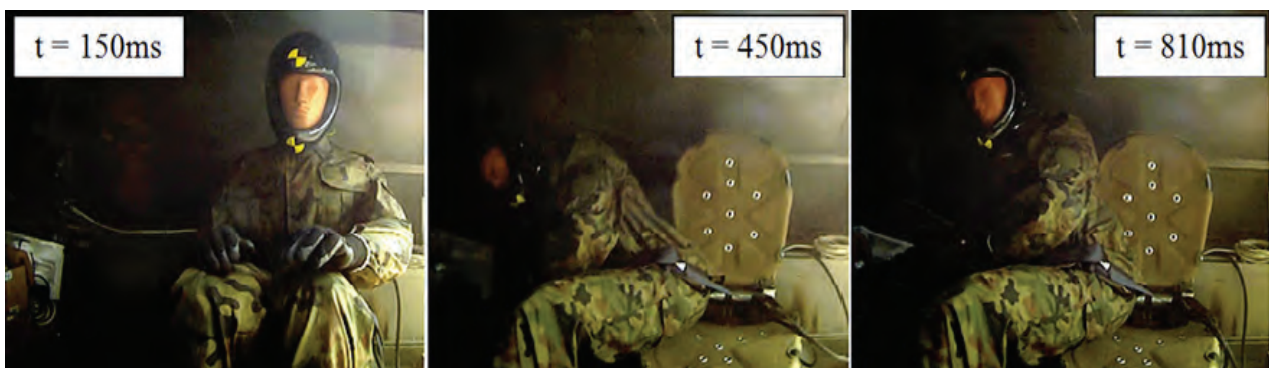
Fig. 7. Phases of motion of the dummy located in the landing troop compartment (trial no. 4)
