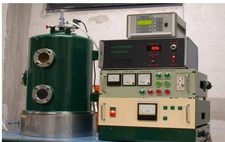
Fig. 1. The view of the system used for deposition of carbon coatings by PACVD method
