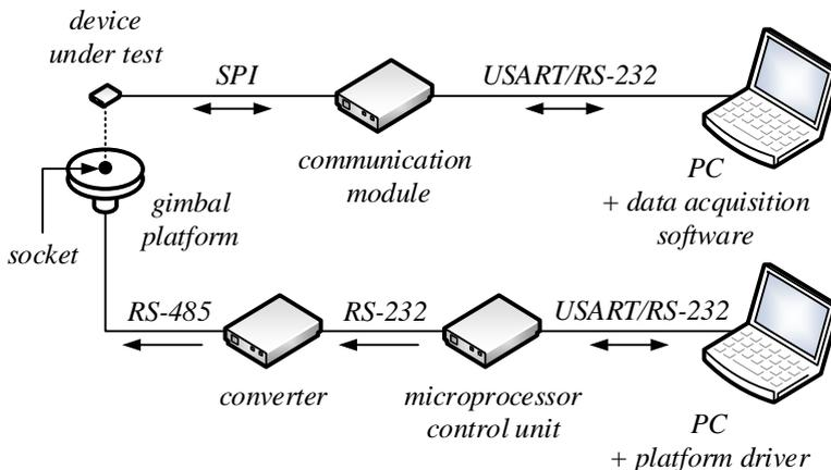
Fig. 4. Block diagram of the laboratory stand
