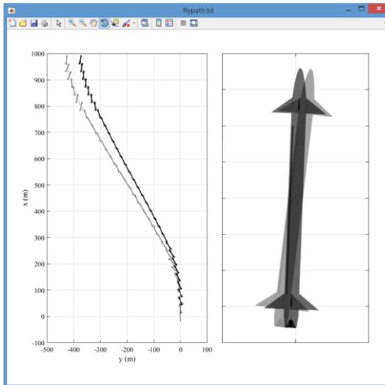
Fig. 8. Missile flight trajectories in the yaw plane
