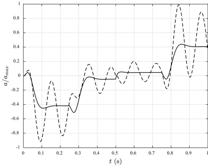
Fig. 5. Normalised accelerations of the missile airframe
