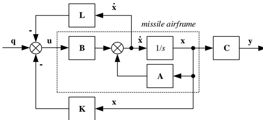
Fig. 2. Block diagram of the dual-control missile stabilization system in the pitch/yaw plane
