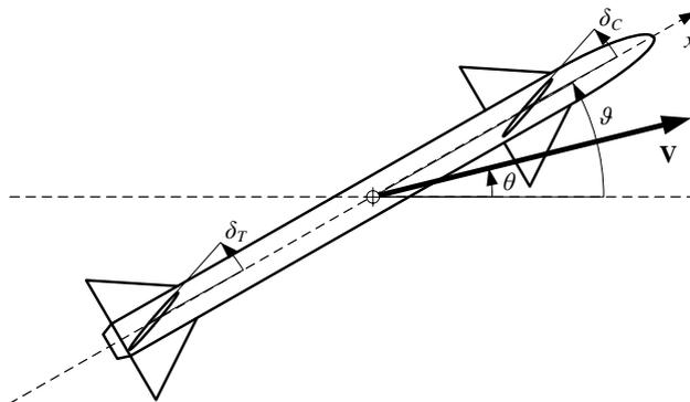
Fig. 1. Dual-control missile configuration
