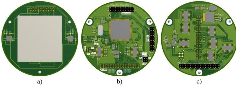
Fig. 3. Elements of the sensor data processing unit: a) AP-01 sensor package, b) AP-02 microcontroller package, c) AP-3 interface package
