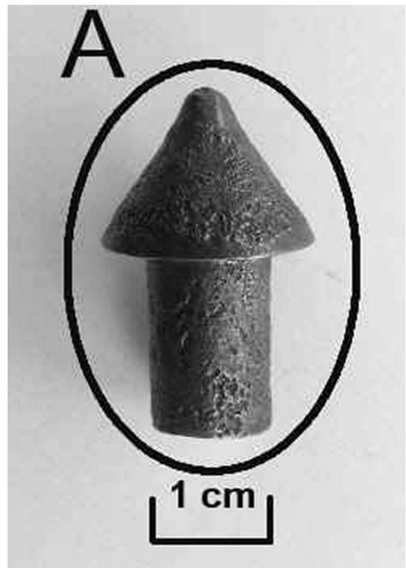
Fig. 12. Investment cast tooth from a working part of the holder
