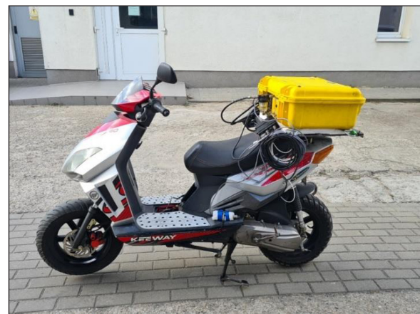
Figure 4. Test vehicle with the AxionR/S+ equipment
