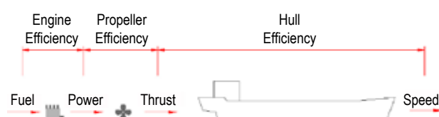
Figure 1. Overall ship efficiency (Cepowski, 2015)
