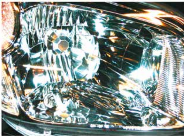
Photo 4. Example of FF headlamp with a double-filament bulb. "Faceted" style
