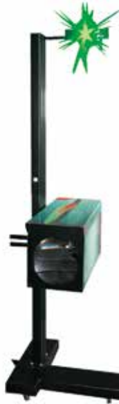
Photo 6. View of a "headlamp analyser"
