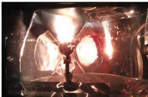
Photo 5. Example of FF headlamp with a single-filament bulb. "Smooth" (continuous-surface) style
