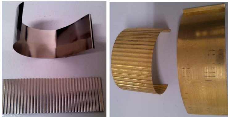
Figure 7. Image of exemplary units of working foils before tests and after 500 START-STOP cycles
