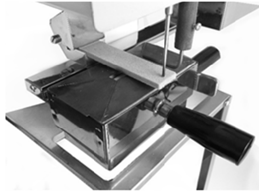
Fig. 4. Hot-distortion test scheme and sample mounted with the lower heating plate placed below [16]
