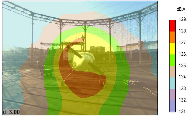
Fig. 6. Noise source distribution of the gyroplane – in front [S. Cieślak, 2016]
