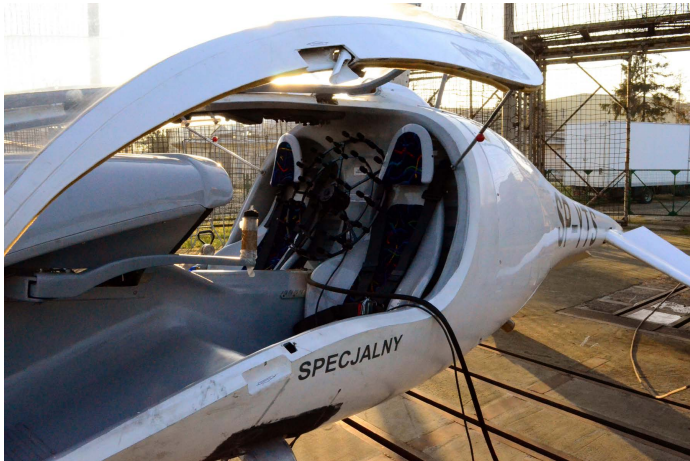
Fig. 8. Acoustic camera set in the gyroplane cockpit [W. Krzymień, 2016]
