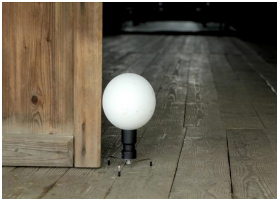
Fig. 5 The marker set on the border of two laser scanned rooms in the door leading from the tower to the nave (photo by Wojciech Markowski)
