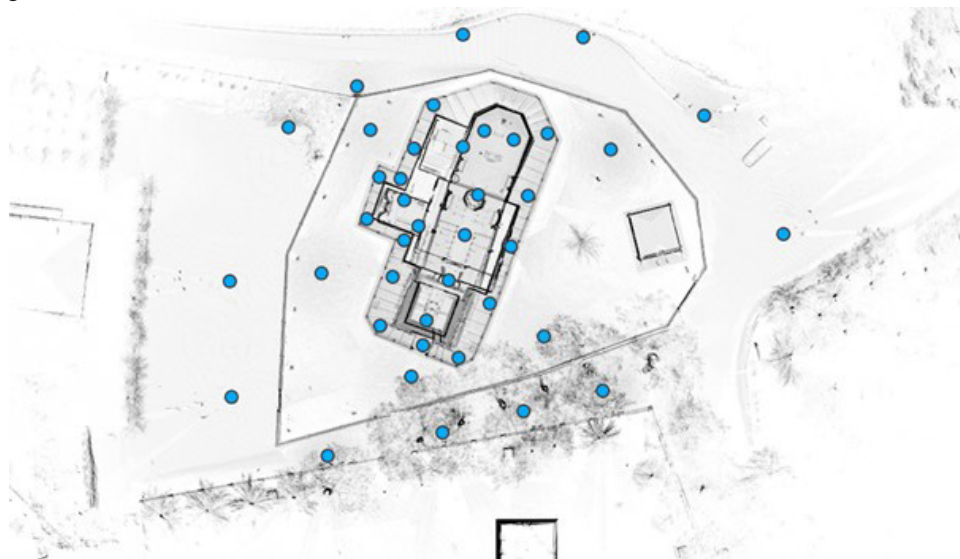
Fig. 4 Top view of the church with marked locations of the scanner (blue dots, image by Wojciech Markowski)
