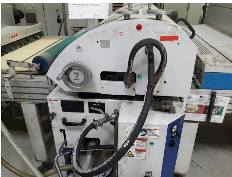
Fig. 1. Roller coater for application of top coating layer
