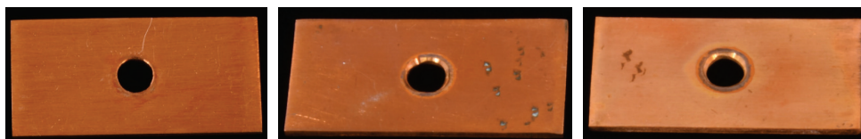
Fig. 2. Macrophotography of plates – on the left - copper plate tested in the original liquid (sample 1), in the middle, the plate tested in sample 3, on the right, the plate tested in sample 2.
