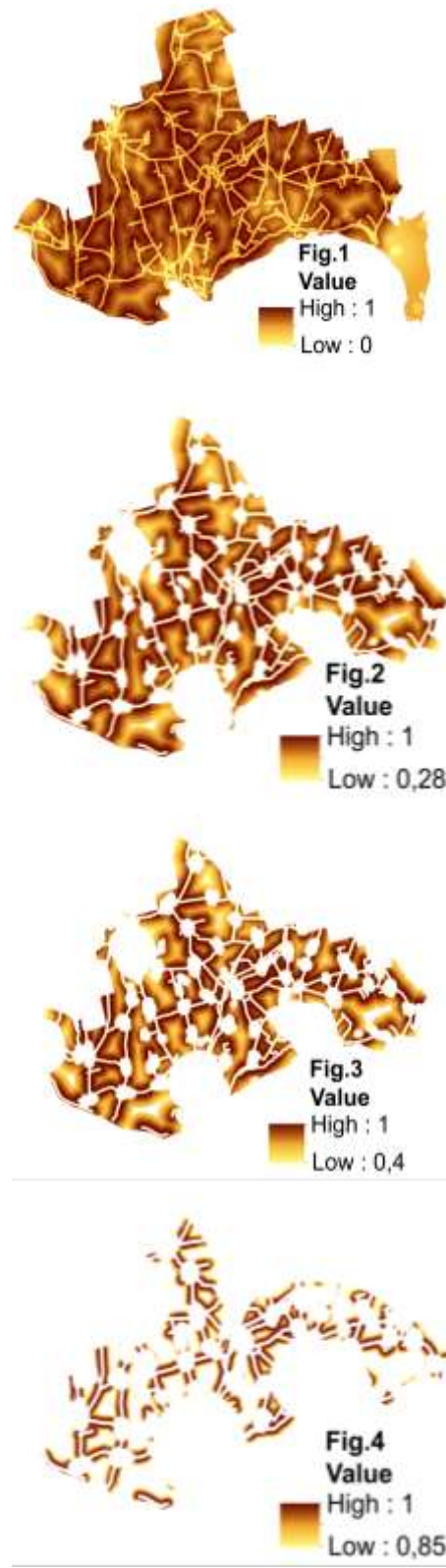
Fig. 5. Combined suitability maps for the placement of a solid waste landfill for different values of \alpha -thresholds of fuzzy sets
