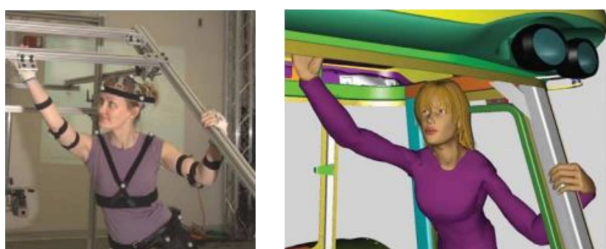
Fig. 7. Virtual reality in assembly process analysis lets verify the reachability to improve the design of product [18].
