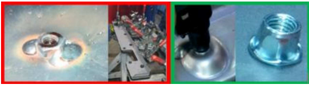
Fig. 13. Comparison between welding nut and rivet nut usage.
