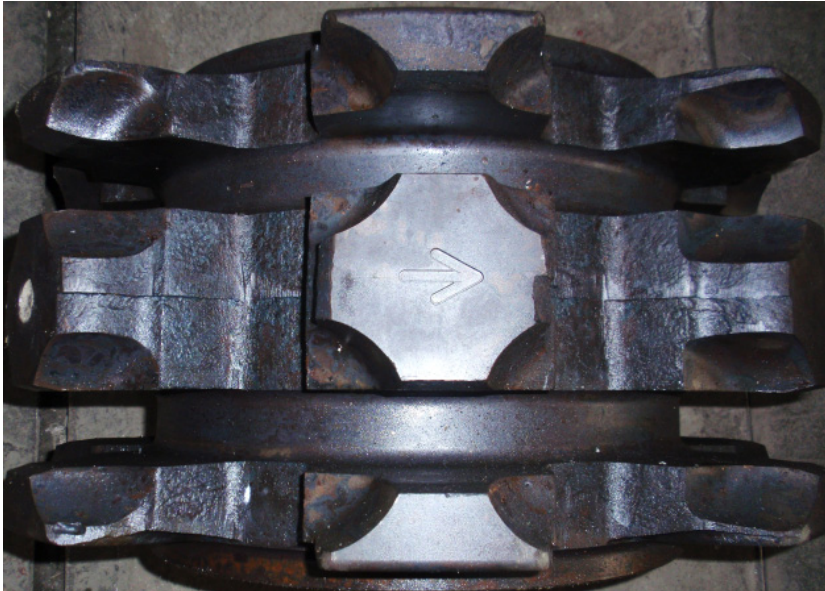
Fig. 11. Drum with the modified profile of seats designed for an armoured face conveyor
