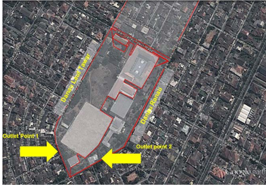
Fig. 2. Outlet point of drainage network at study area; source: own elaboration based on field survey & Google Earth
