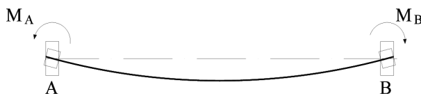
Fig. 6. Emerging of reaction bending moments in bearings
