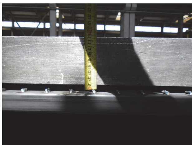
Fig. 4. A view of an element during measuring a deflection after a couple of minutes from the end of the test ( f=6 mm)
