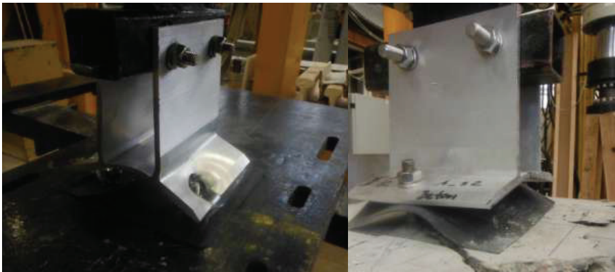
Fig. 5. Damaged aluminium brackets after tensile tests
