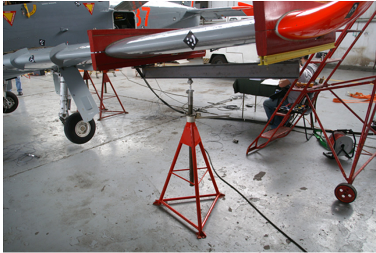
Fig. 15. Calibration of strain gages – loading of the wing
