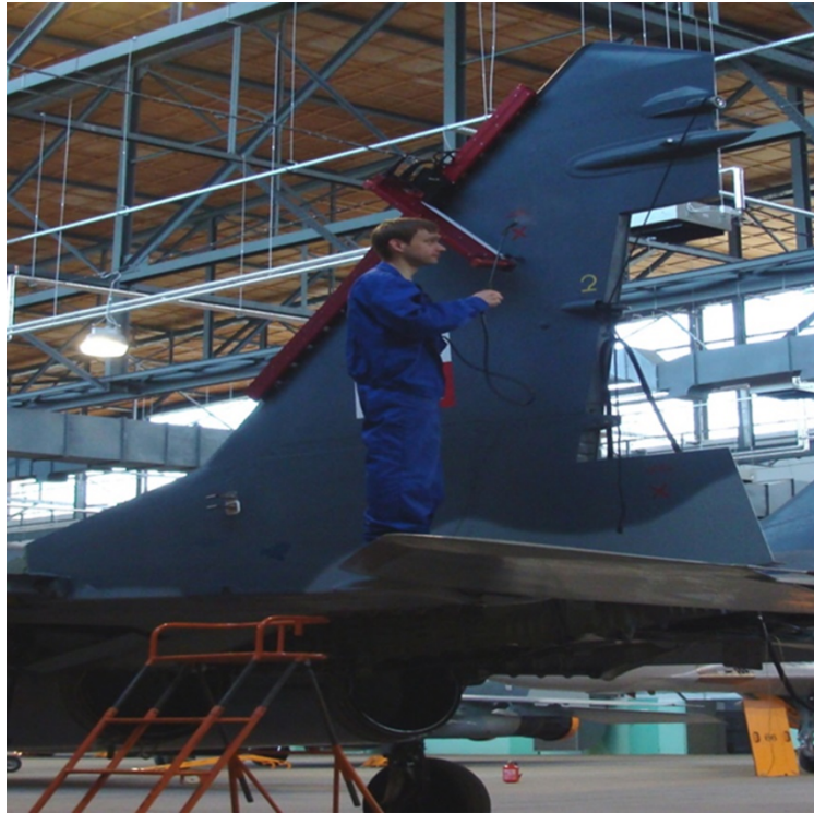
Fig. 3. Composite Vertical Stabilizer Inspection
