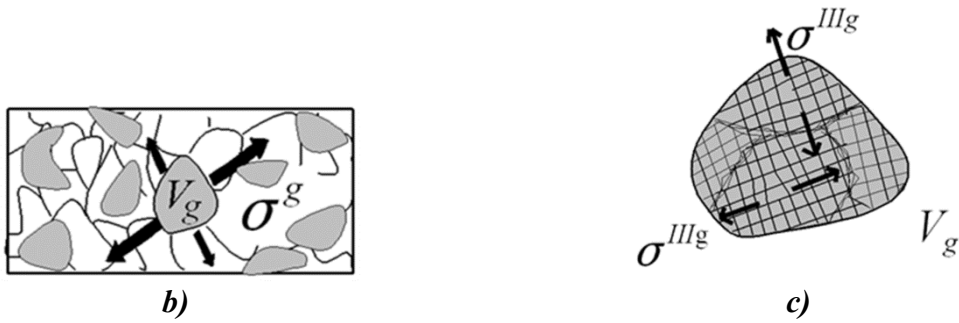
Fig. 27. Stress classification: a) first order stresses, b) second order stresses, c) third order stresses
