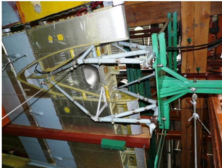
Fig. 7. PZL M28 05 wing and wing load carry-through structure fatigue test fixture. The engine frame is loaded by vertical power plant inertia force, engine torque and balancing prop thrust force.
