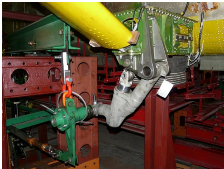
Fig. 6. PZL M28 05's wing and wing load carry-through structure fatigue test fixture.
