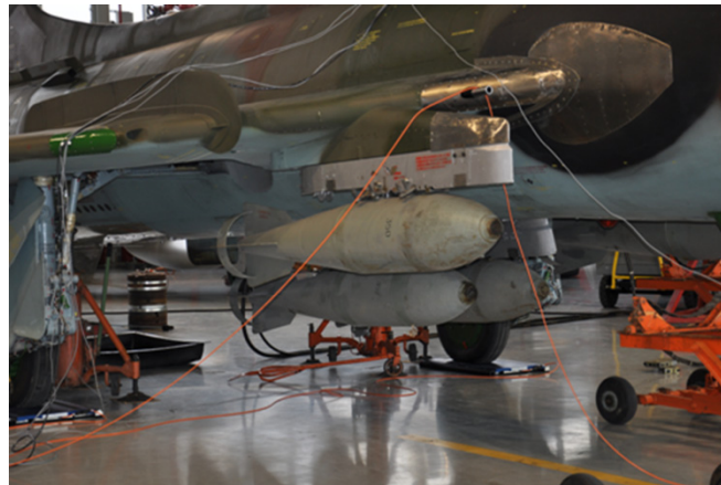
Fig. 13. Scaling of strain gauges – loading of the fuselage
