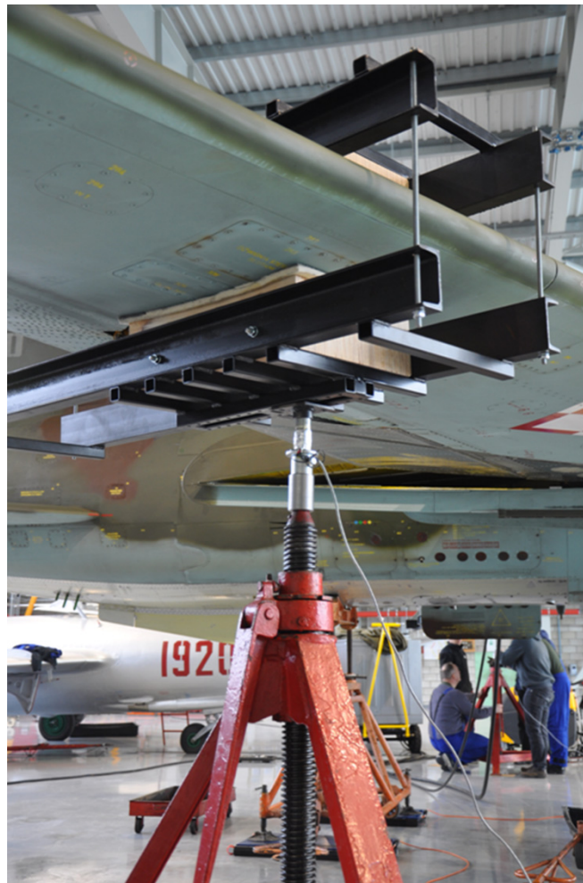
Fig. 12. Scaling of strain gauges – loading of the wing
