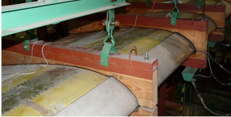
Fig. 4. PZL M28 05's wing and wing load carry-through structure fatigue test fixture. Clamps introducing loads to the wing are shown.
