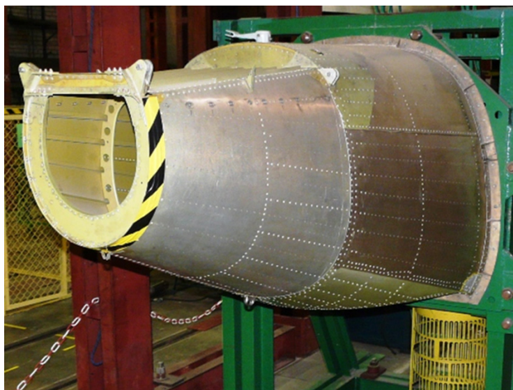
Fig. 8. PZL M28 05's empennage fatigue test fixture. In the picture there is a fuselage part used in test (empennage is dismantled).
