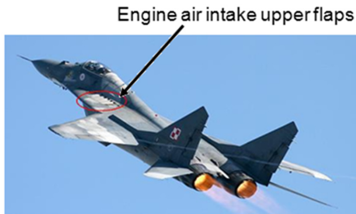
Fig. 10. Location of the engine air intake upper flaps
