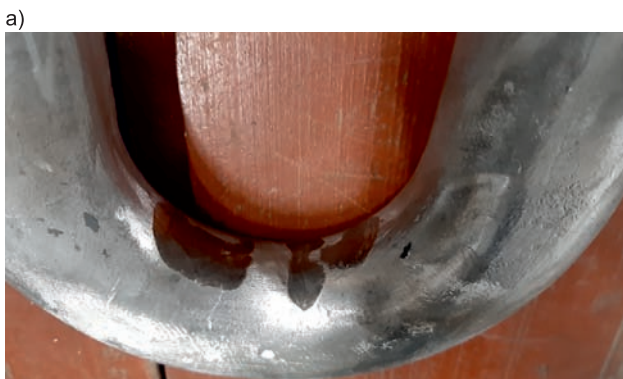
Fig. 5. View of the worn coupling bow surface caused by friction with the draw hook: a) left view, b) right view [pic. D. Kowalczyk]
