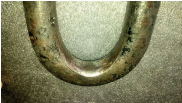
Fig. 1. View of the worn (in operating conditions) surface of the bow caused by abrasion against the draw hook [pic. A. Aniszewicz]
