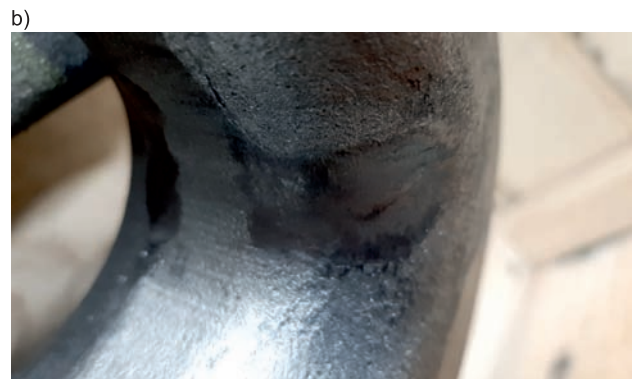
Fig. 5. View of the worn coupling bow surface caused by friction with the draw hook: a) left view, b) right view [pic. D. Kowalczyk]
