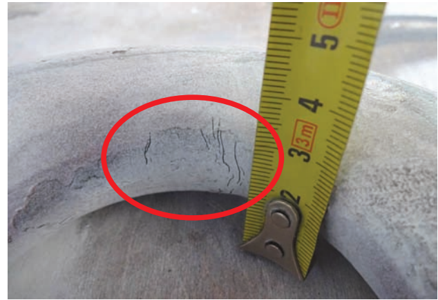
Fig. 4. Cracks in the 1 MN bow after fatigue testing using the magnetic particle inspection [pic. D. Kowalczyk]
