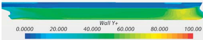
Fig. 2. Y+ value on hull surface
