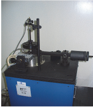
Fig. 1. Tribological tester T-11 used in the laboratory tests
