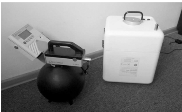
Fig. 4. Instruments used for AIM. The Berthold LB125 UMo with LB6411 neutron tube on the left and RSS131 ionisation chamber on the right.
