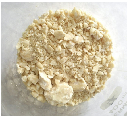
Figure 11. A typical granulate of the washed out TNT particles is in the form of “semolina”
