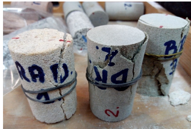
Figure 6: Cracked samples after uniaxial compression test.
