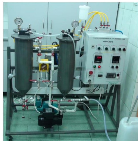
Fig. 3. Reactor GW 200 for production of Biodiesel FAME (SME)
