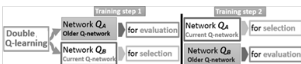
Fig. 16. Double DQN use 2 Networks QA and QB that switch their roles after each training step
