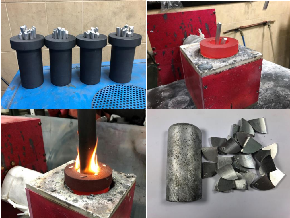
Fig.2. Stages of the Al-Cu-Mg metallurgical synthesis (a-pure aluminium, b –melting a batch in an induction furnace, c – refining of the liquid metal, d – ingot and samples taken for testing from Al-Cu-Mg alloy). Source: Authors'
