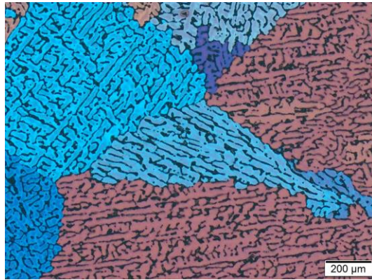
Fig. 8. Microstructure of AlCu4.5Mg6 alloy before modification. Source: Authors'
