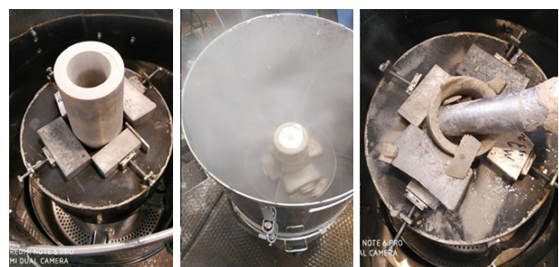
Fig. 3. Modified ablation casting process steps; Lukasiewicz Research Network – Krakow Institute of Technology [17]
