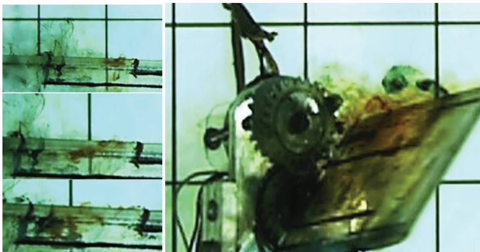
Fig. 6. Spanwise flow of LEV
