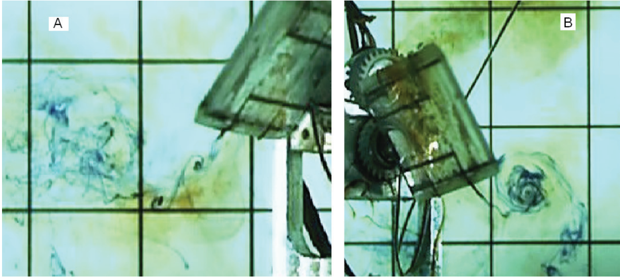
Fig. 7. Trailing edge vortex and starting vortex for reduced frequency 0.15 (A) and 0.4 (B)
