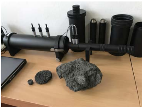
Fig. 10. Measuring stand with lava rock samples.
