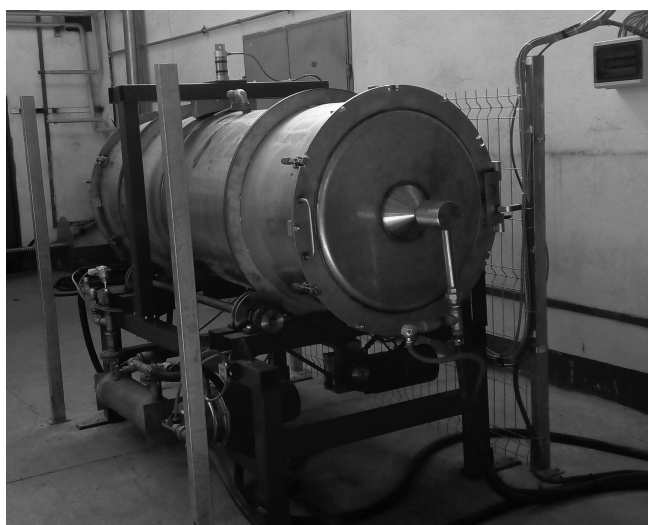
Figure 2. Closed device with liquid flow (rate of water flow 30 l/min) produced by the Institute for Sustainable Technologies, Radom.
