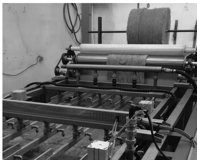
Figure 3. Degumming in an open devices with water and ultrasound. Batch size: 4.5 m x 1.5 m x 0.6 m, produced by the Institute for Sustainable Technologies, Radom.
