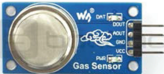
Figure 2. MQ-135 Carbon dioxide sensor (8)
