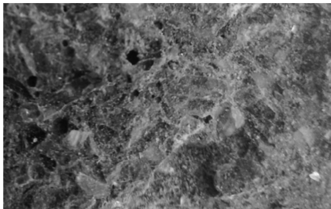
Figure 7. Breakthrough of a composite sample containing flint after compressive strength testing
