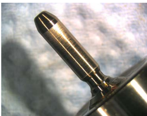
Figure 16. Friction and corrosion wear of the control valve piston (Common Rail)
