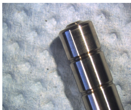
Figure 17. Friction and corrosion wear of the knife-edge follower (Common Rail).
