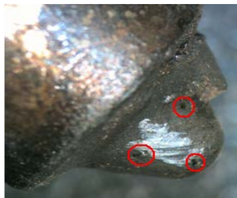
Figure 10. Overheating and change of the structure of the Common Rail-Bosch sprayer ending
