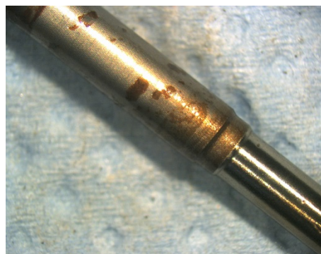
Figure 15. Corrosion pits on the needle which affected by sulphur and water compounds in fuel
