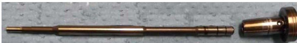
Figure 13. Wear of the surface of the needle valve of Common Rail injector
