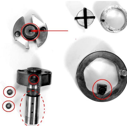
Figure 5. Selected elements of the injection pump DPA by CAV which are subject to intensive wear during exploitation
