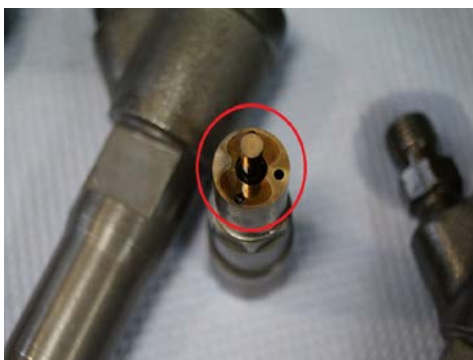
Figure 14. Corrosion pits on the injector sprayer which occurred affected by sulphur and water compounds in fuel
