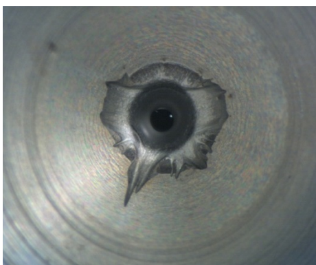
Figure 11. Damage to the control valve set of Common Rail-Bosch
