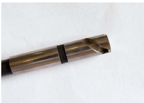
Figure 1. Plunger from Motorpal pump of Zetor tractor after 3000 motohours of operation
