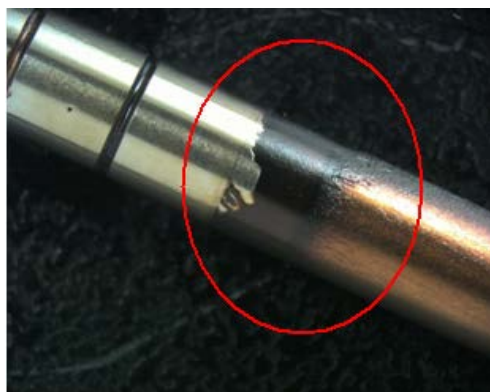
Figure 9. Corrosion pits on the knife-edge follower from Common Rail -Bosch sprayer
