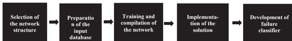
Fig. 1. Diagram of the procedure for the development of a short-circuit detection system
